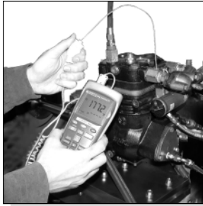
Testing the temperature at the discharge fitting.
