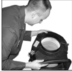
Inspect the engine air cleaner.
