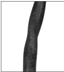
Partly collapsed inlet line shown.
