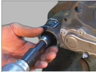
Figure 68 – Remove the Caliper Bolts
