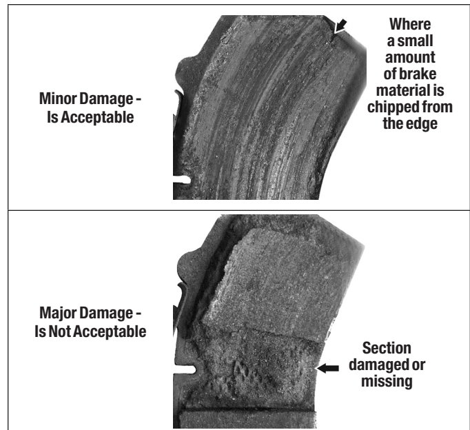
Figure 24 – Brake Pad Surface Inspection
