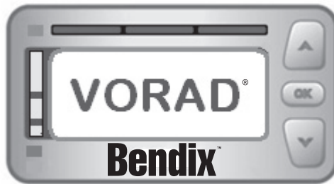
VS-400 DIU Lamp Test at initial power-up
