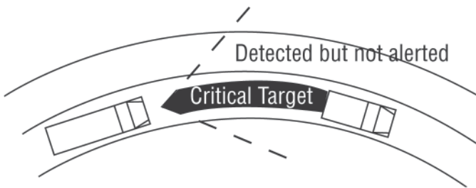
Vehicle tracking in a curve.
